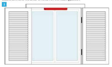
This function is activated just when the sensor is in the HORIZONTAL position and afterwards it is inclined. In order to activate the removal detection, it is necessary to put the sensor horizontally: from now on the anti-removal is activated; if the sensor moves it indicates tamper alarm.
