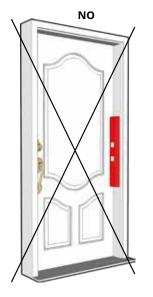
The detector must be installed with the side that presents the LEDs towards OUTSIDE (garden, backyard, balcony...) and the opposite side towards INSIDE (door or window) to protect:
