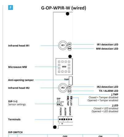
It is recommended to disable the LEDs (J.LED = OPENED) after the test.
