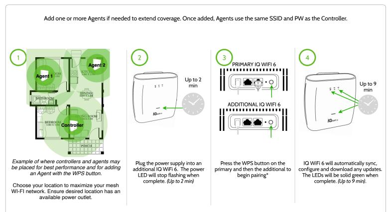
Please note: Ethernet backhaul is supported when you plug an ethernet cable between LAN to LAN. A switch may be needed for more than two IQ WiFi 6's. IQ WIFI6 will default to a WiFi backhaul if no physical LAN connection is made between routers.
