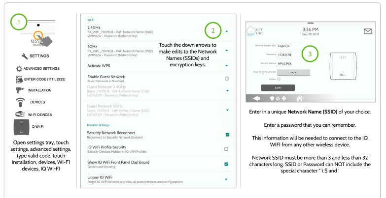
\*Note: IQ WIFI6 supports band-steering. This setting can not be disabled, so when you edit the 2.4GHz SSID or encryption key these changes will also effect the 5GHz settings to be the same as well. (profile name, mesh name, user device name, password): disallows " \ and \$
