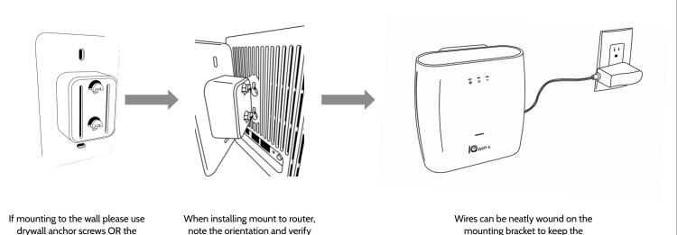
drywall anchor screws OR the provided sticky tape on the mounting bracket. Verify that the mount provided is oriented with the space in the tab UP.
