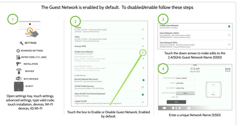
\*Note: Guest network can be disabled from the IQ WIFI Front Panel Dashboard as well. Enabling/disabling the guest network will reboot the router (will take ~5 seconds before the panel will show that the router has disconnected for reboot)
