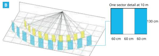
Each detection head is equipped with a Fresnel lens that builds 5 sectors, each divided in a couple of beams (fig. B-1)
