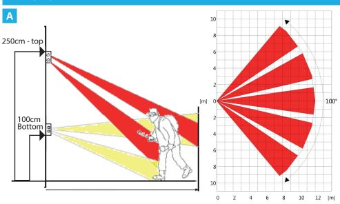
Installation height of the center of the sensor must be between 100cm and 250 cm(fig. A1) The detection arear is max 12 meter long and 100° wide (fig. A-2)
