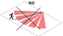
To obtain a reliable detection, it is recommended to mount the detector in the way that the intruder crosses beams perpendicularly and not with frontal approach (fig. **D**).
