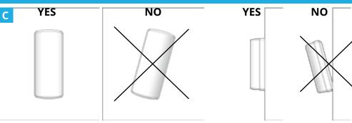
Mount the sensor vertically, without front or side inclination (fig. **C**): the joint of each IR head allows to adjust the orientation.
