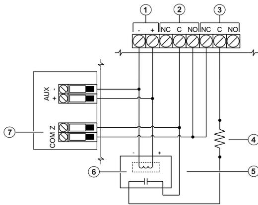
**Figure 10: 4-wire smoke and heat detector wiring**
